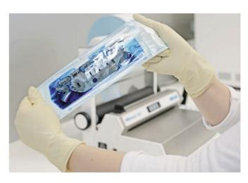
The MELA*ink* test is a reliable test for performing a weekly routine check of the seal seam for leaks in accordance with DIN EN ISO 11607-1 and ASTM F1929-12.
