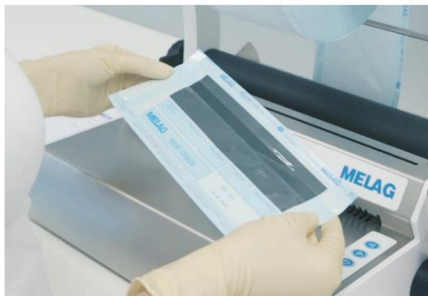
The **daily MELAcontrol Seal Check** verifies the quality of the seal seam in accordance with DIN EN ISO 11607-2.
